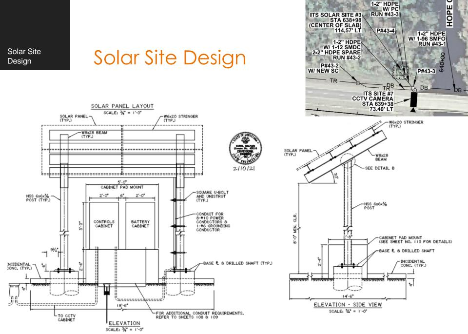
Note: NFPA 855-20 "Installation of Stationary Energy Storage Systems" may apply to the site design. The standard does not apply to lead-acid battery installations less than 70 kWh storage capacity. MUTCD latest edition and NESC may have applicable standards as well depending upon the site location.
